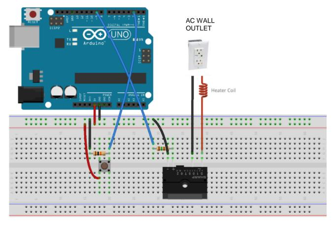
If you have used the same GPIO pins, there will be no code changes required to operate the solid-state relay. You should be able to trigger the relay simply by pressing the push-button.
