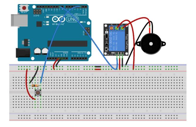
Pressing the button shall activate the relay, and the buzzer shall sound with its characteristic beeping sound. Interfacing the relay to the Arduino using the ready-made module illustrated above is as easy as interfacing an LED, (or even easier, since there are no resistors needed) and operating it is as easy as writing HIGH to the appropriate pin.
