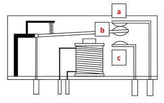
When there is adequate power applied to the electromagnet / coil, it generates a magnetic field which forces the armature to switch position, linking the contacts together, or breaking contact, depending on the relays' construction.
